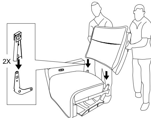
**STEP 2** : Attach the ① to the ④ with the connectors.
