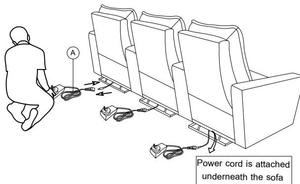
**IMPORTANT NOTE :** PLEASE ENSURE THAT ALL ELECTRICAL CORDS AND CABLES ARE CLEAR OF THE FRAME AND MECHANISM. FAILURE TO DO SO MAY SEVER YOUR POWER CORD RESULTING IN SERIOUS INJURY OR DEATH.
